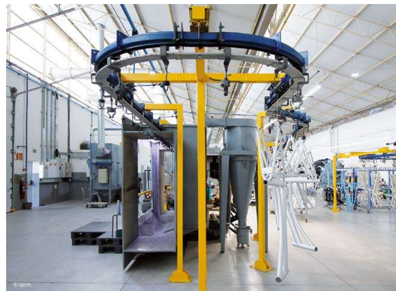
One of the three bicycle assembly lines and the powder coating plant.
