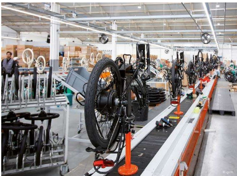
One of the three bicycle assembly lines and the powder coating plant.
